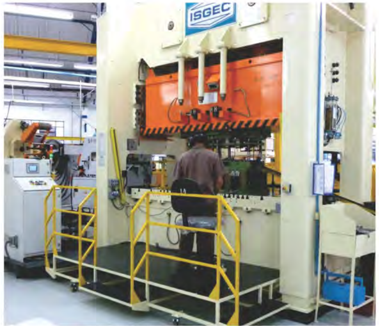
315 T MAX 2L Press supplied for Progressive Die Application
