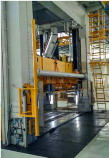
Automatic Swing Arm assembly duly interlocked with Slide Movement Photoelectric Guards & Two Hand Run Button Station for Operator Safety
